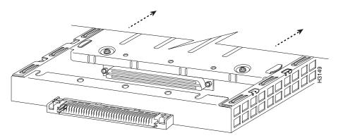
Step 7 If you removed a port adapter, place it in an antistatic container for safe storage or shipment back to the factory. If you removed a blank port adapter, no special handling is required; however, store the blank port adapter for potential future use.
